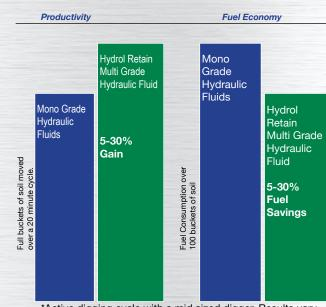
\*Active digging cycle with a mid sized digger. Results vary depending on equipment, hydraulic oil and test conditions.
